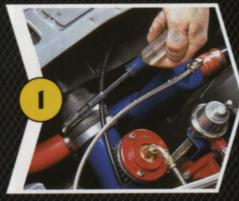
The intercooler is located beneath and protrudes from the slam panel. Undo the retaining clips on each of the hoses that connect the intercooler to the turbo and throttle elbow, and squeeze the hoses to free them before pulling them clear.
