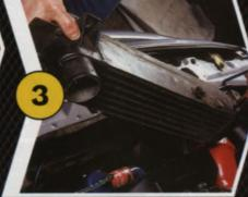
Undo the two bolts which secure the intercooler and radiator through the same fixing holes. The radiator need not be removed or disconnected, but must be loosened. The old unit can now be discarded.
