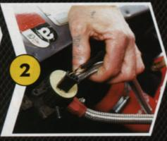
Remove the two self tappers that secure the amal valve to the top of the intercooler. That's amal valve, with an 'm' ...
