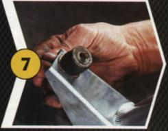
The larger Pace item also has additional fixing brackets for which you need rubber mounts and two new bolts of the same size and thread as the top two. No additional drilling is required on the three-door Sierra, as the shell is identical to the RS500 which was fitted with a larger intercooler as standard, so the chassis rail is pre-drilled.
