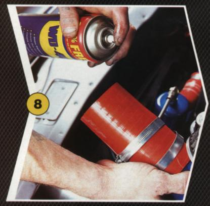
With the big intercooler now securely bolted into position, it's simply a case of refitting the hoses and the amal valve.
